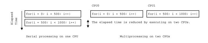
Although the elapsed time will usually decrease with multiprocessing, the total CPU time required to execute the program may increase. This is because the total CPU time is at least as large as the CPU time when the program is executed on a single processor, and the overhead time for multiprocessing may increase the total CPU time.
