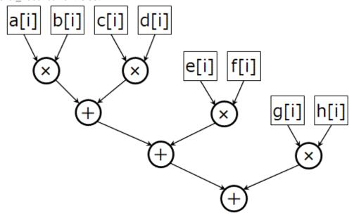
Figure 3.4 The calculation tree when the -Keval\_concurrent option or optimization control specifier eval concurrent is set
