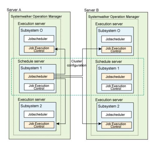
In the example in the following figure, Subsystem 1 on Server A is used as a schedule server, while Subsystem 1 on Server B and Subsystem 1 on Server C are used as an execution server in a cluster configuration, and Subsystem 0 on Server B and Subsystem 0 on Server C are used as independent execution servers.
