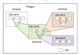
In this example, job net A is in the first level, job net B is in the second level, and job net C and job net D are in the third level. Job net A is the parent of job net B. Job net B is the parent of job nets C and D. Job net B is a child of job net A, and job nets C and D are children of job net B.
