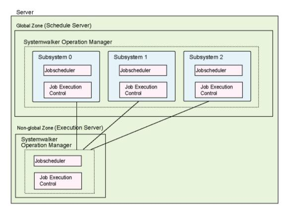
Systemwalker Operation Manager runs by regarding each zone as a single server. Even for multiple subsystem operations, network jobs can be submitted from a subsystem in a zone by assigning logical IP addresses to the zones and specifying logical port numbers for the multiple subsystems.
