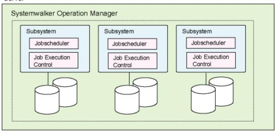
If multi-subsystems operate on a single machine, subsystem 0 can be used for production system operations, subsystem 1 can be used for testing next month's data, and subsystem 2 can be used for testing new jobs, for example.
