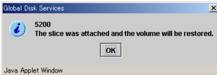
Figure 7.45 Notifying Attach Slice Completion
