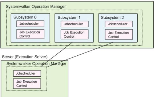
Operating multiple subsystems consisting of only schedule servers makes it possible to perform test operations that link to network jobs, as shown in the following example.
