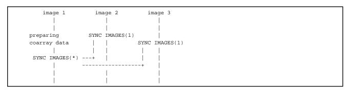
The correct result is obtained without synchronization between images 2 and 3 because it is required that images preparing data, image 1, should synchronize with images using data, images 2 and 3.
