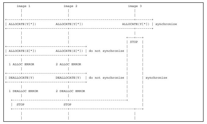
The first ALLOCATE statement is executed on all the images correctly. The second ALLOCATE statement is executed on images 1 and 2 while the STOP statement is executed on image 3. Then, the variable specified with STAT= specifier in the ALLOCATE statement on images 1 and 2 is set to the STAT\_STOPPED\_IMAGE.
