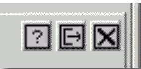
Figure 110: Detail of tab view showing detach button
