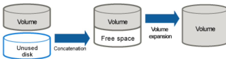
Figure 1.24 Concatenation and Online Volume Expansion
