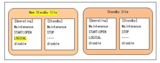
6. Confirm whether the logical standby database is ready to switch to the primary database. Issue the following SQL statement on a new logical standby database.
