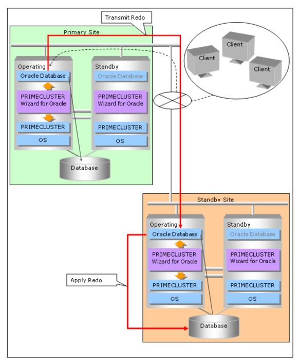
In the standby operation using Oracle Data Guard, the operation node and the standby node exist on the primary site and the standby site. Oracle Database operates in the operation node of each site. In the event of a failure, userApplication is switched to the standby node, and the resources in this standby node become activated.
