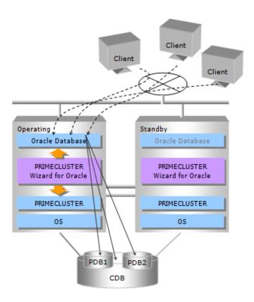
The multitenant configuration is supported by the standby operation or the single-Node Cluster operation. The starting, the stopping and the monitoring of CDB are the same as Oracle instance. After CDB is started, PDBs are started. When fault of PDBs is detected, the message is output to syslog. The restart and the failover due to fault of PDBs is not executed.
