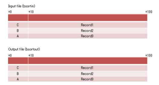
bsortex -copy -record recform=fix -input reclen=100 file=bsortin filesys=dos -output file=bsortout filesys=cobs64
