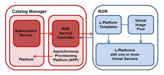
In CT-MG, customer subscriptions are managed by means of the **Subscription service**. When a customer creates, modifies, or terminates a subscription for a virtual system in ROR, the Subscription service asynchronously triggers the corresponding actions in ROR through the **Asynchronous Provisioning Platform (APP)** and the **ROR service controller**: Virtual platforms or servers are created, modified, or deleted in ROR.
