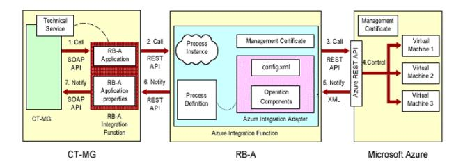
The installation flow for a process instance of RB-A to become available as a CT-MG service using the Azure integration function and RB-A integration function is shown below.
