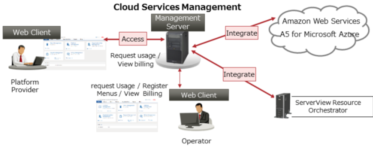
Figure 1.2 System Configuration of Cloud Services Management
