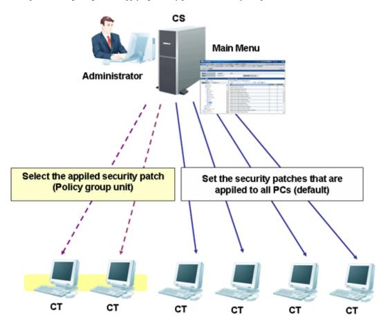
For the PC that does not belong to the policy group, patch application can be performed according to the security patch settings selected in the **Distribution** > **Distribute Security Patches** window.
