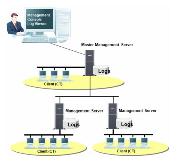
3-Level System Structure (with Virtual Environment)
