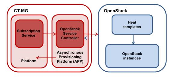
In CT-MG, customer subscriptions are managed by means of the **Subscription service**. When a customer creates or terminates a subscription for a virtual system in OpenStack, the Subscription service asynchronously triggers the corresponding actions in OpenStack through the **Asynchronous Provisioning Platform (APP)** and the **OpenStack service controller**: Virtual systems are created or deleted in OpenStack.
