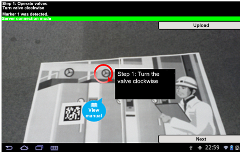
Figure 7.2 Example overlay for operating valves
