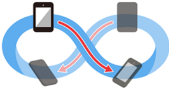
Figure 1.2 Adjusting the geomagnetic sensor
