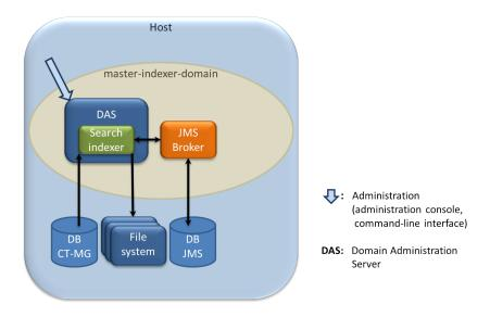
Host is the machine where your application server is installed. The master-indexer-domain domain has a Domain Administration Server (DAS) which is used for domain administration and the hosting of the search indexer application. Data for indexing is read from the CT-MG database
