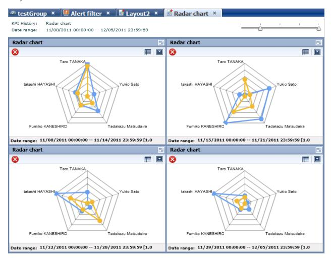
History shows a list of charts for the period selected with the period slider. View each period side by side for a simple comparison. Adjust the period displayed by moving the slider at the top of the window.
