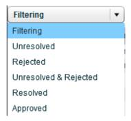
The displayed alert list can be filtered according to the alert status by using the **Filtering** list located at the top of the alert list. You can select multiple alerts and process them collectively.
