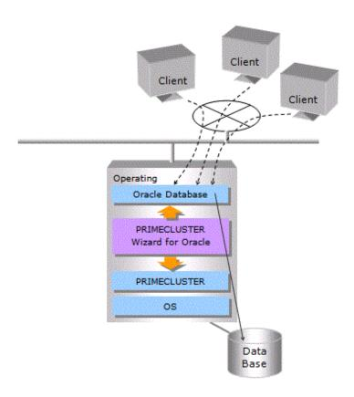
In Single-Node Cluster operation, a cluster system consists of one node.
