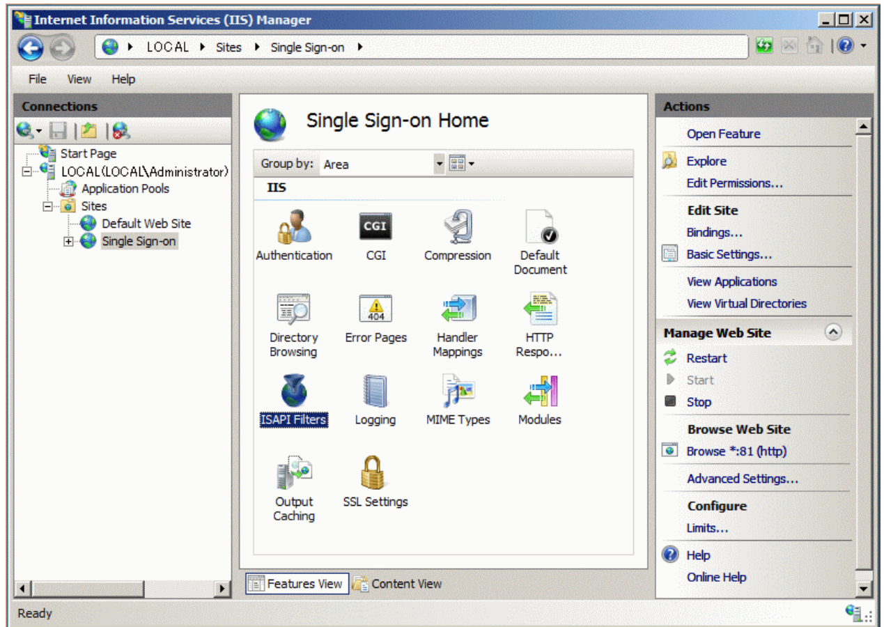
Figure 3.30 Open the Virtual Directory Creation Wizard window
