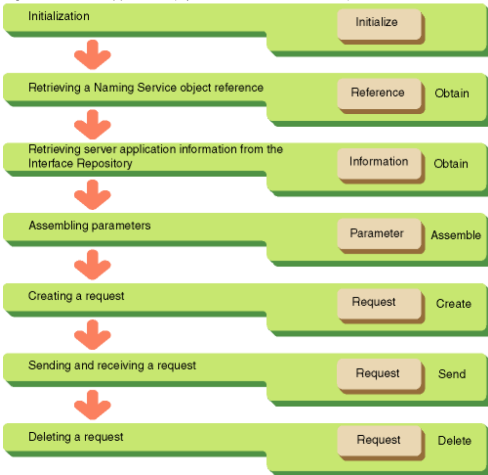
Figure 7.2 Client Application (Dynamic Invocation Interface) Process Flow
