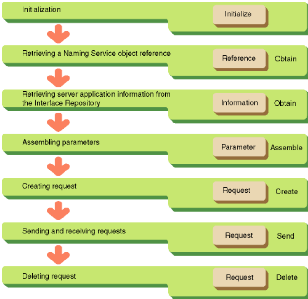
Figure 4.2 Client Application Processing Flow (Dynamic Invocation Interface)
