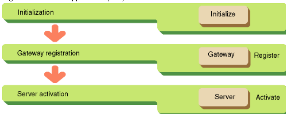
Figure G.3 Server Application (DSI) Process Flow
