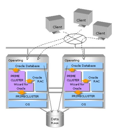
In scalable operation with Oracle9i RAC or Oracle RAC 10g, Oracle is operated on all nodes. The clients can access to the database regardless of which node they are connected to.
