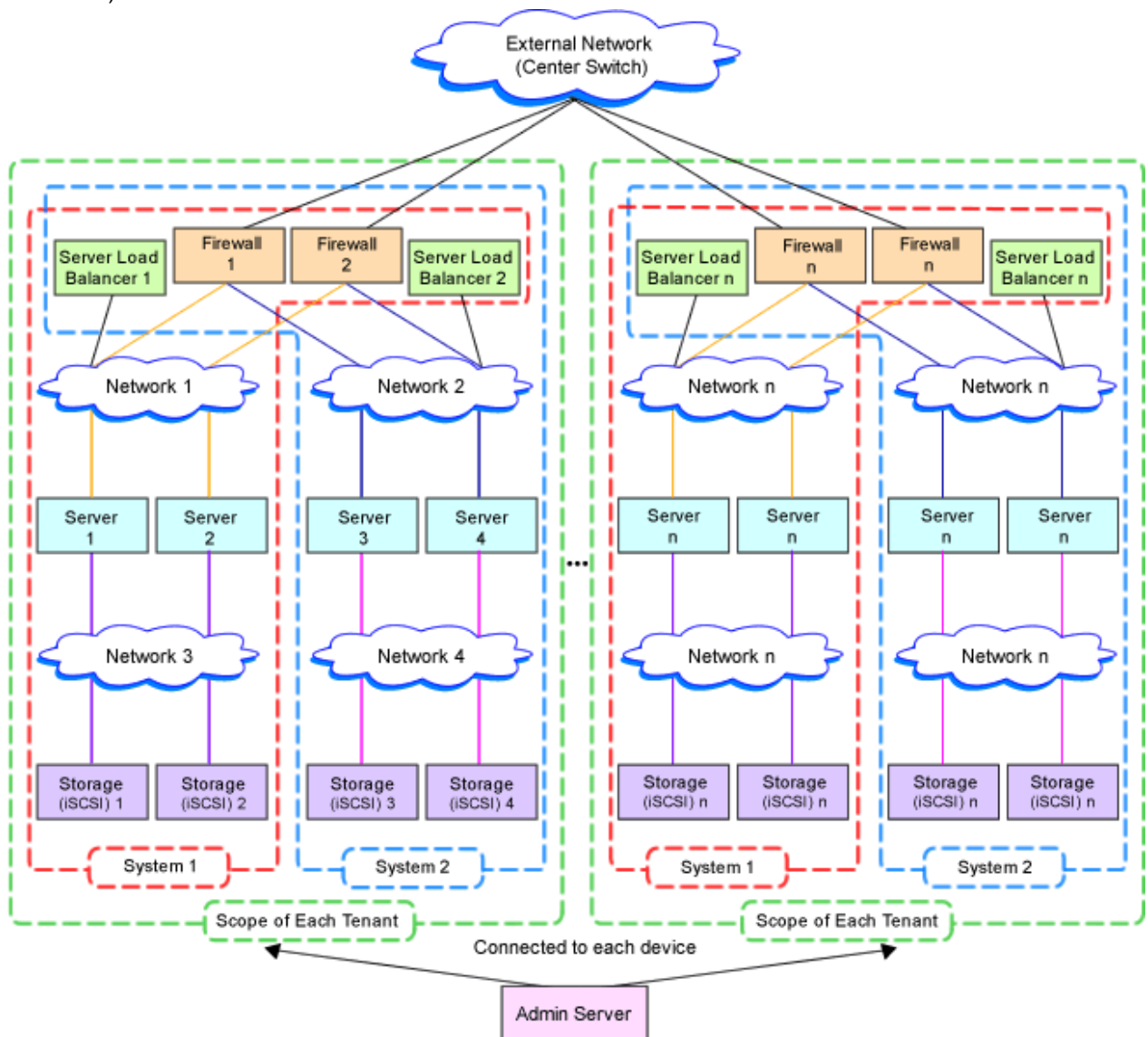
Figure 9.6 Example of Overall Configuration of a Virtual System (A Collective of Virtual System Configuration Elements)
