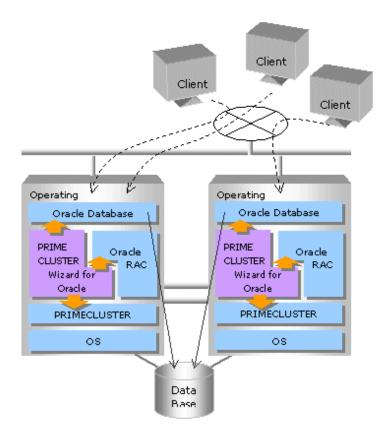
In scalable operation with Oracle RAC, Oracle is operated on all nodes. The clients can access to the database regardless of which node they are connected to.
