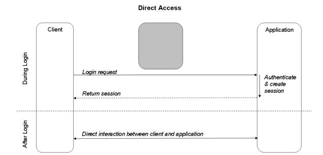
The following figure shows the interaction between the client, BSS, and the application:
