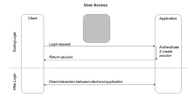
The following figure shows the interaction between the client, BSS, and the application:
