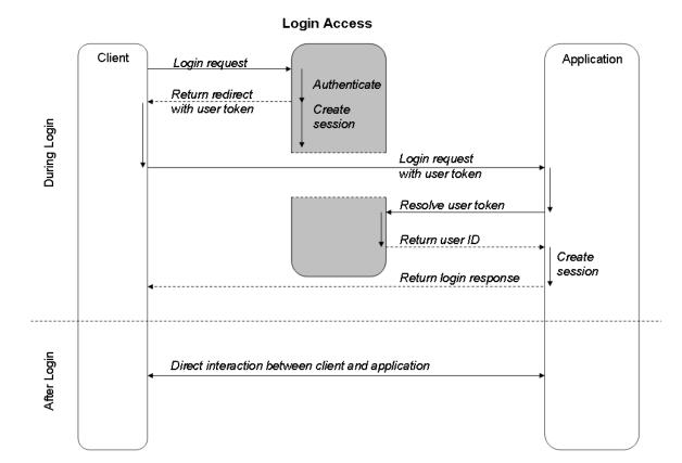
The following figure shows the interaction between the client, BSS, and the application:
