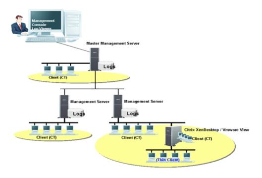
3-Level System Structure (with Log Analysis/Report Output and Citrix XenApp Monitoring)
