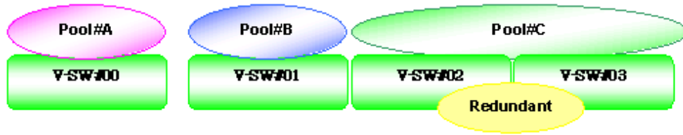
Figure F.3 Image of specifying virtual storage pools and virtualization switch groups
