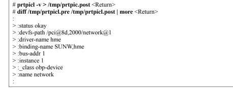
b. It confirms that the interface name that obtained above-mentioned procedure is an interface name that corresponds to the PCI bus slot of the added PCI card.
