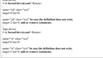
b. In case /kernel/drv/sd.conf was updated in 1.a., reconfigure the kernel , restart the system, and then start system operation.
